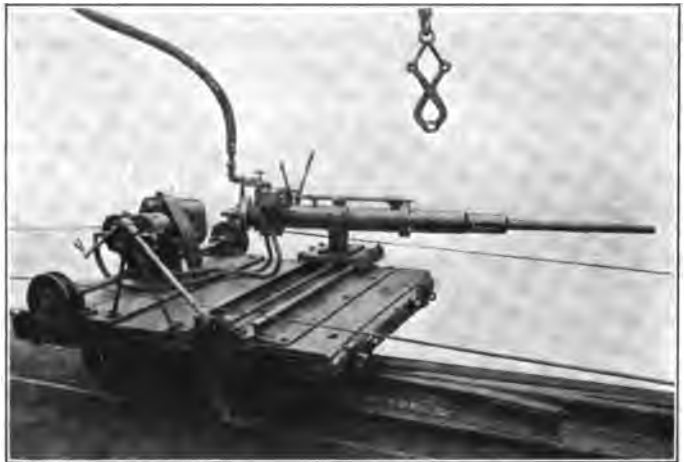
Machine for Breaking Rivets In Frogs at the Dover Shops of the Lackawanna.
