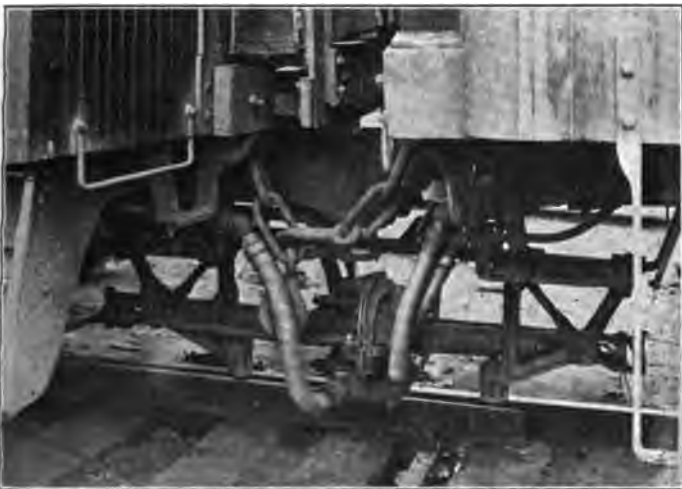
Durbin Automatic Train Pipe Connector as Connected in Service.
