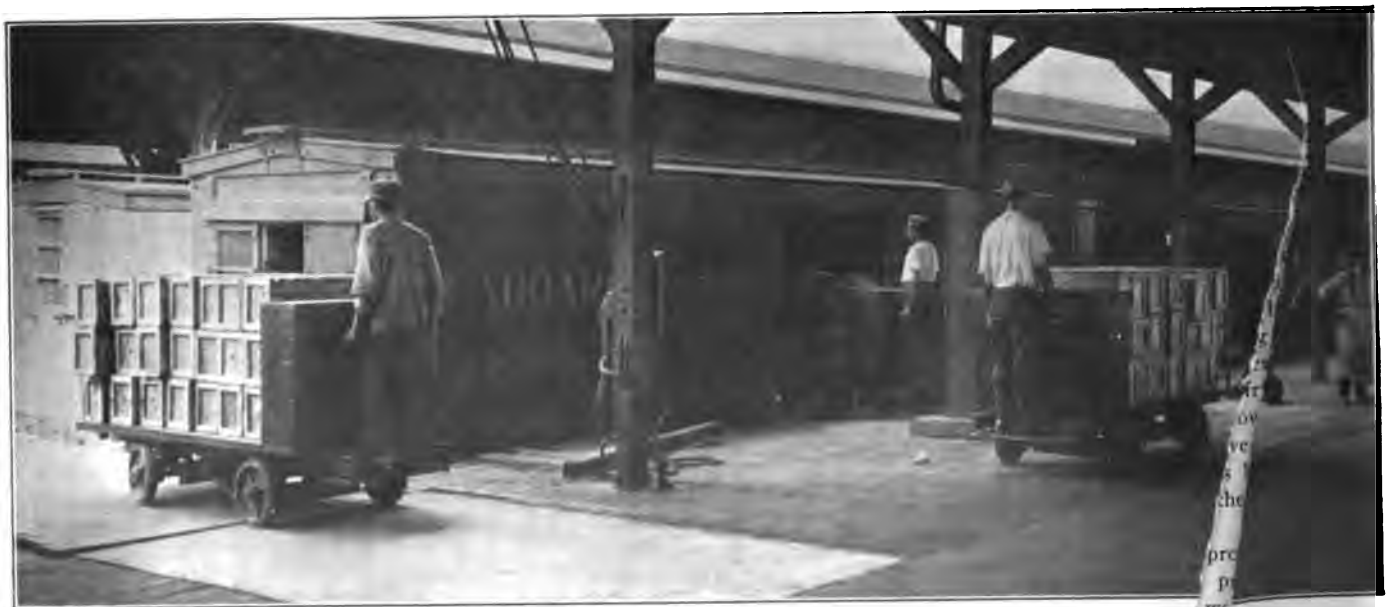
Electric Trucks Used in Loading Cars on Merchants' & Miners' Transportation Pier at Savannah, Ga.
