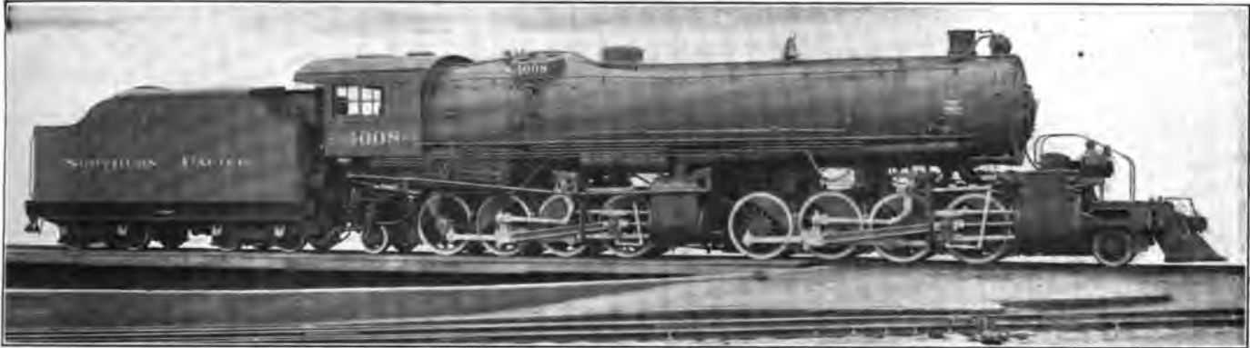
Powerful Articulated Pusher Locomotive; Northern Pacific.
