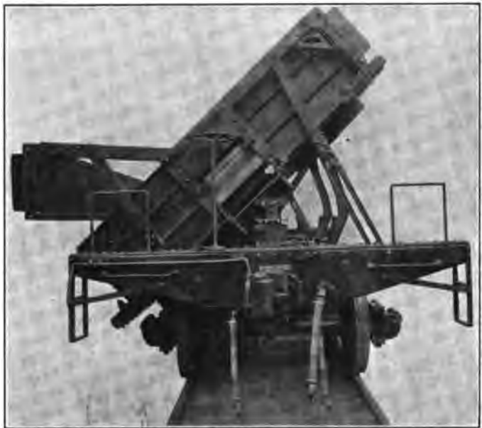
End View of Steel Air Dump Car, Showing Hinged Doors, etc.
