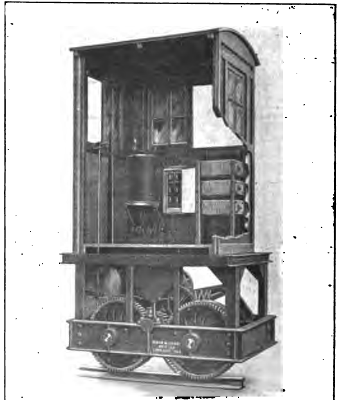
Fig. 4—Arrangement of Apparatus on Turntable Tractor.
