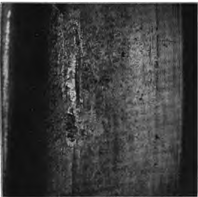
Thermal Cracks on Face of Tire at Outer Edge of Tread.
