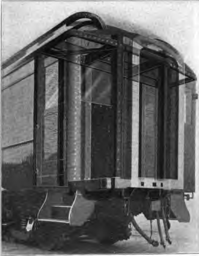
New End Construction for Both Steel and Wooden Cars.
