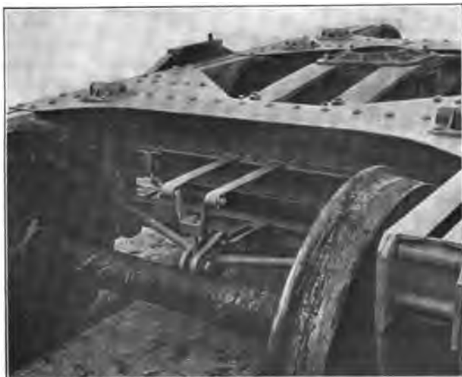
End View Showing the Brake Beam Adjuster and the Absence of the End Piece.
