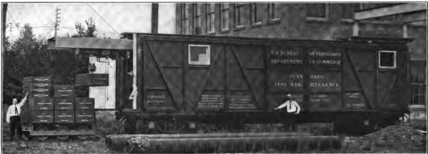
Scale Test Car of U. S. Bureau of Standards.
