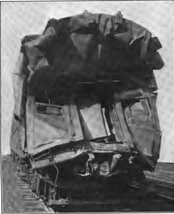
Showing How the End of the Steel Parlor Car Was Crushed In at the Tyrone, Pa., Wreck.
