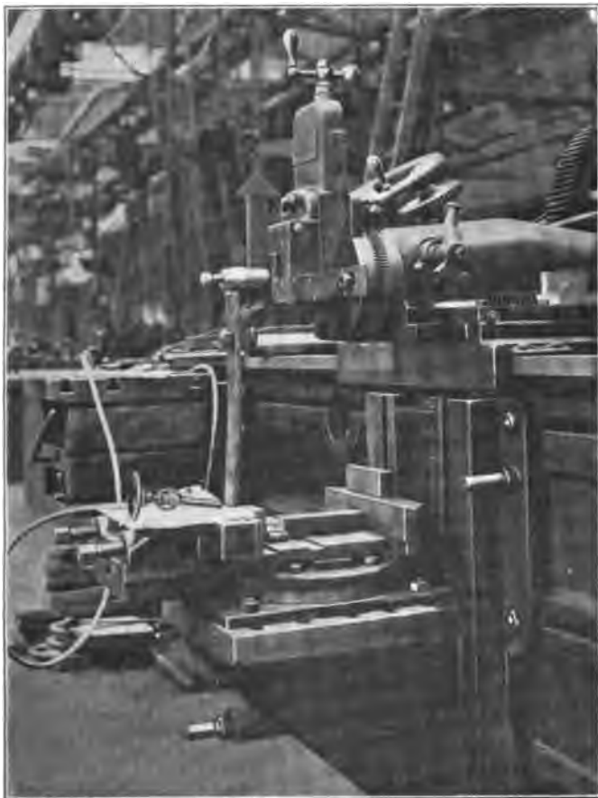
Fig. 3—Shaper Arranged for Vibrating Test of Firebox Steel.
