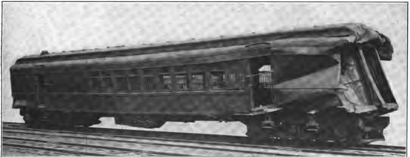
The Crushing of the End of this Steel Car Absorbed the Shock and Protected the Body of the Car.
