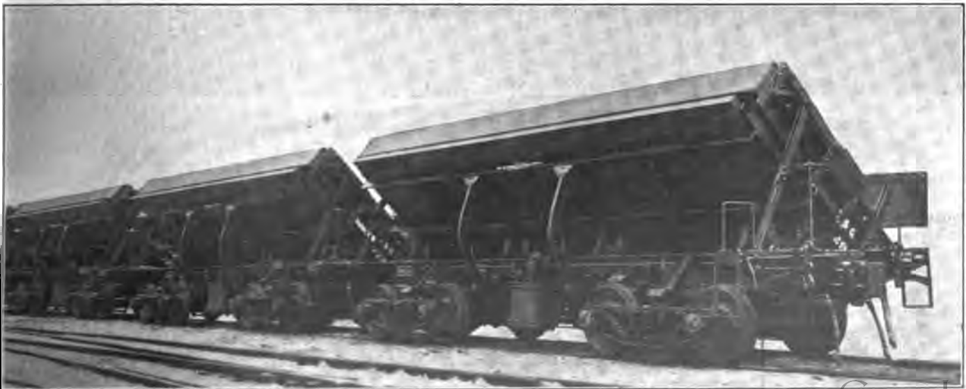
Under-side of Dump Cars, Showing Air Cylinders and Operating Mechanism.
