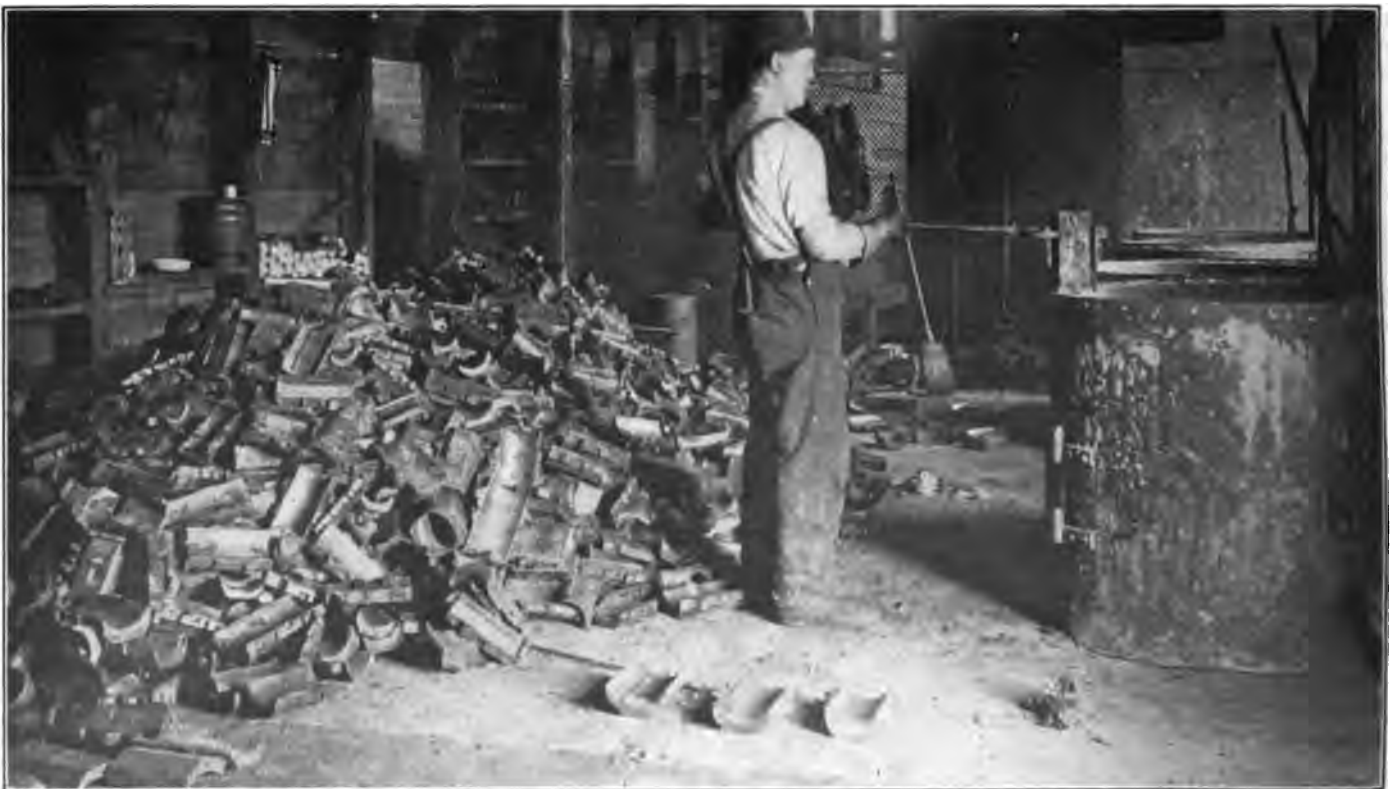
Fig. 17—Reclaiming Babbitt from Old Car Brasscs at Corwith
