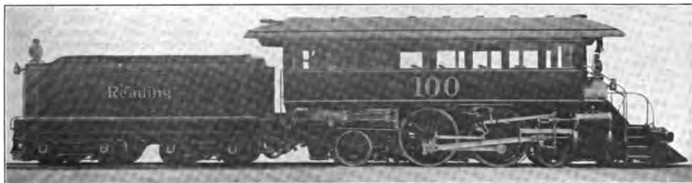
Atlantic Type Inspection Locomotive Designed and Built by the Philadelphia & Reading.
