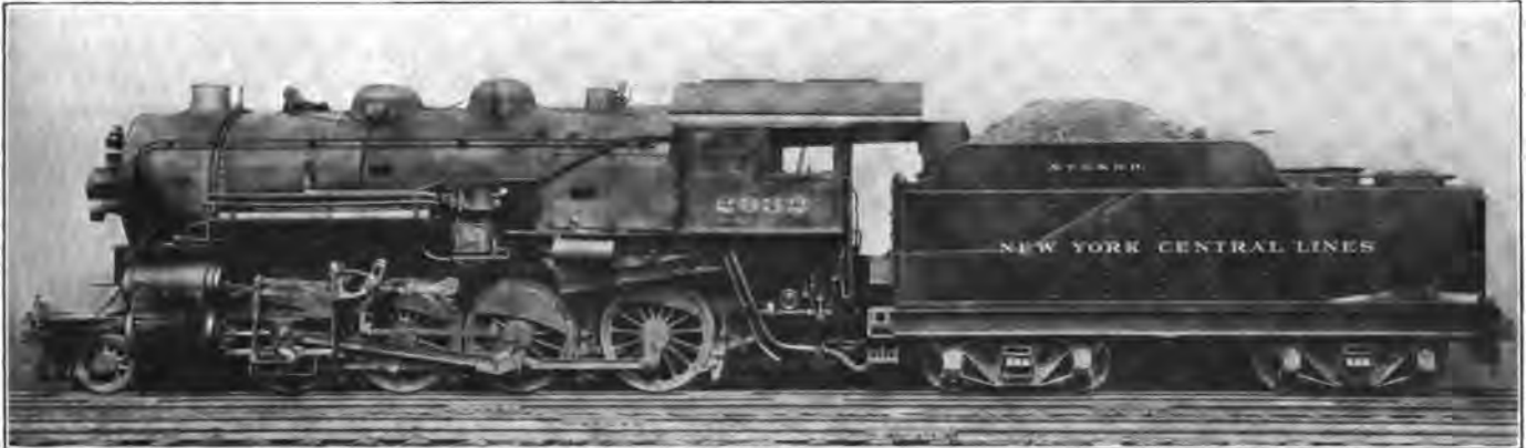
Class G 6 F Consolidation Locomotive, New York Central, Fitted with a Standard Stoker.
