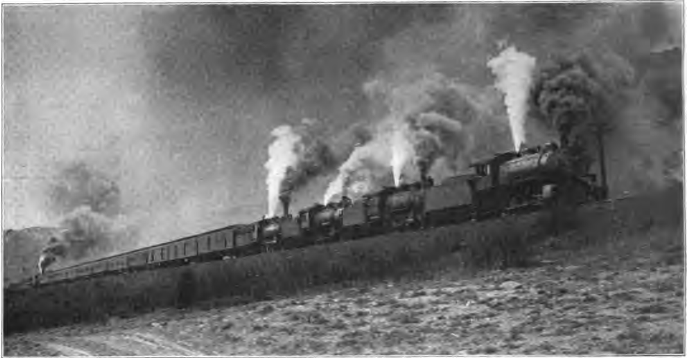
Train No. 6 Eastbound on April 26, 1911, Ascending Four Per Cent. Grade with Five Engines Pulling Eleven Cars.
