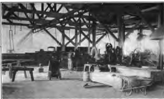
View in Frog Erecting Shop Showing Riveting Benches and Finished Products Storage.
