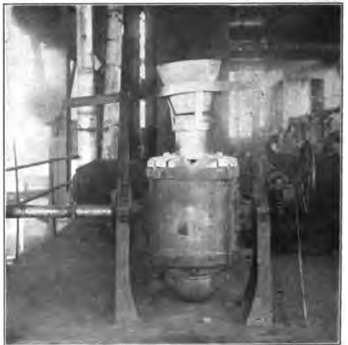
Tilting Brass Furnace of 400 lbs. Capacity.
