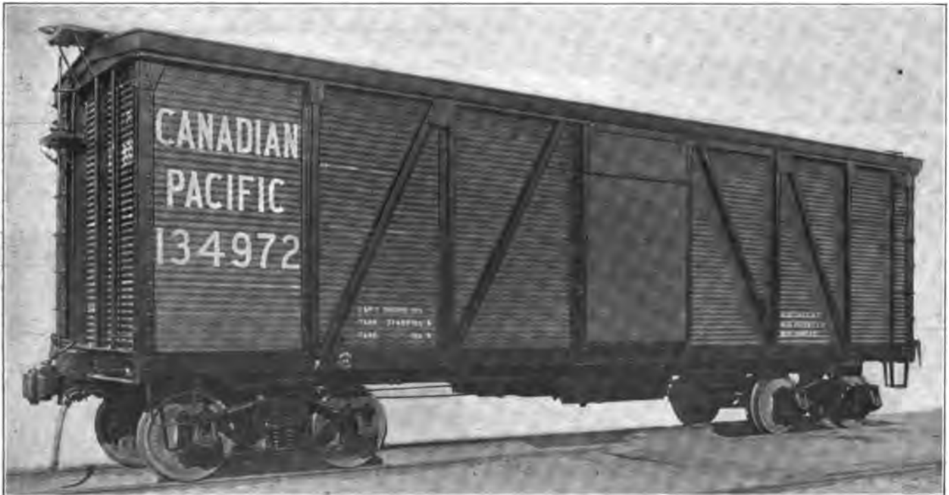
Canadian Pacific Steel Frame Box Car with Corrugated Metal Sheathing.
