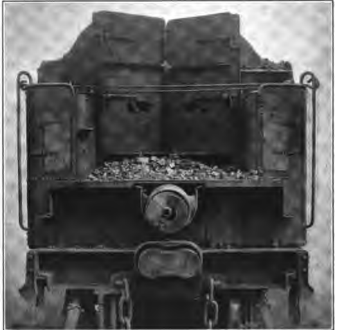
View of the Tender Showing the Location of the Conveyor.
