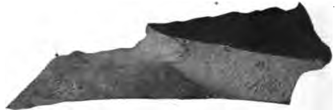
Piece from Wheel Broken in Testing, Showing the Structure of the Metal.
