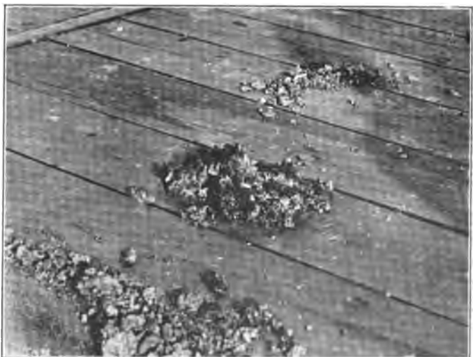
Result of Test on Missouri River Bridge, Showing Slight Charring of Wood.
