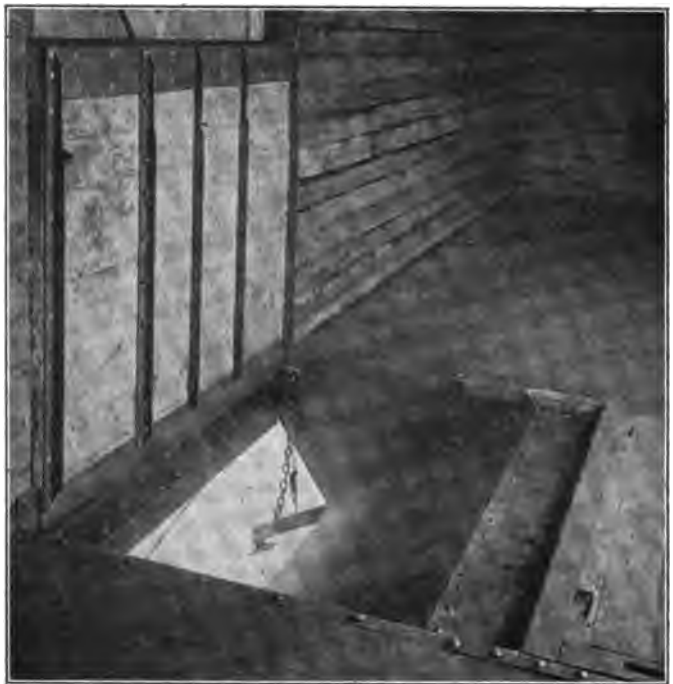
Interior of Box Car Showing Grain Door and One Open Hopper.
