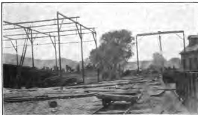
Portion of Scrap Yard Showing Frogs Held for Breaking up in Foreground and Scrap Bins in Background.
