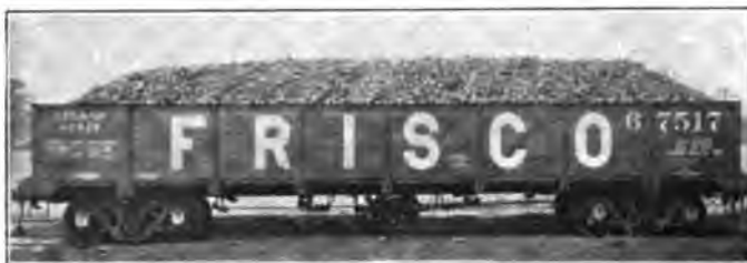
Properly Loaded 50-Ton Gondola Car; Net Weight, 107,500 lbs.
