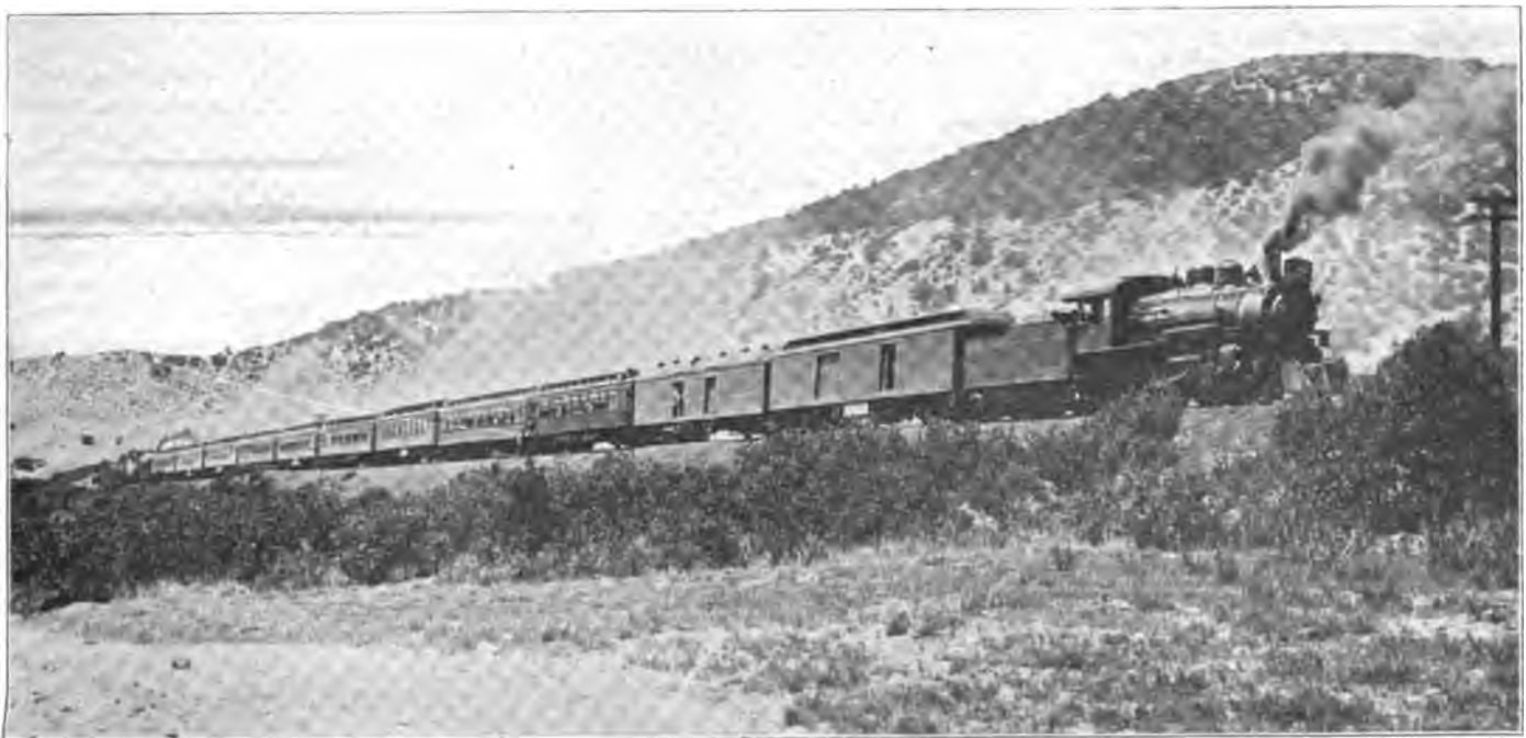
Train No. 6 Ascending Four Per Cent. Grade with One Road Engine and a Mallet Pusher on July 10, 1913.
