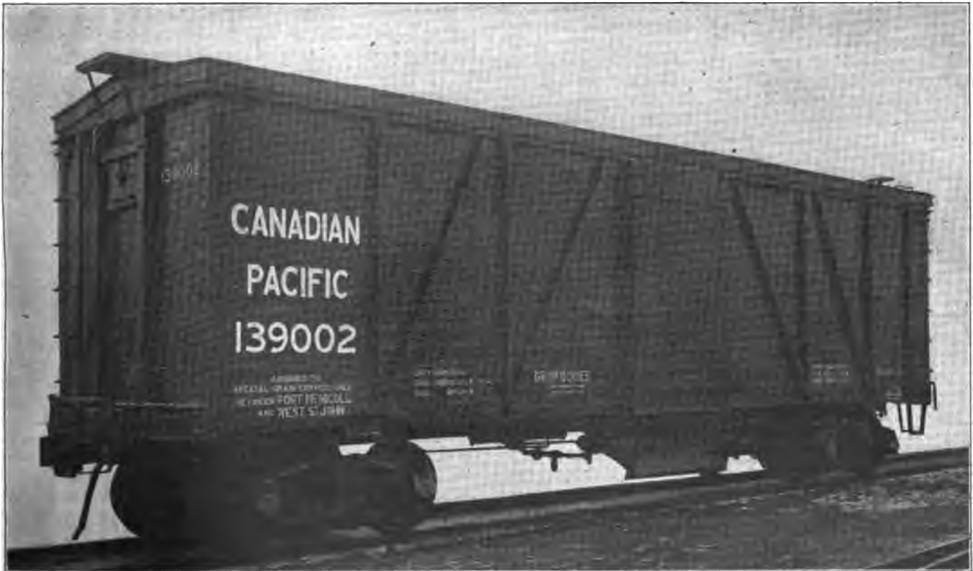
Canadian Pacific Hopper Bottom Box Car for Grain and Coal Traffic.
