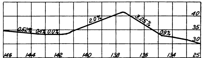
Profile Over Hump in C. M. & St. P. Air Line Yard.
